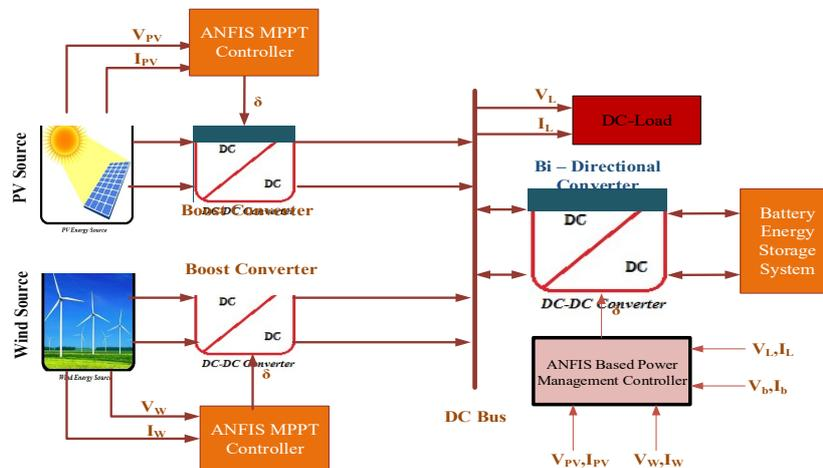
Fig.1 Basic Topology of the Proposed Hybrid System
