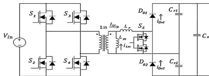
**Fig. 9. Isolated Bidirectional DC-DC Converter**
