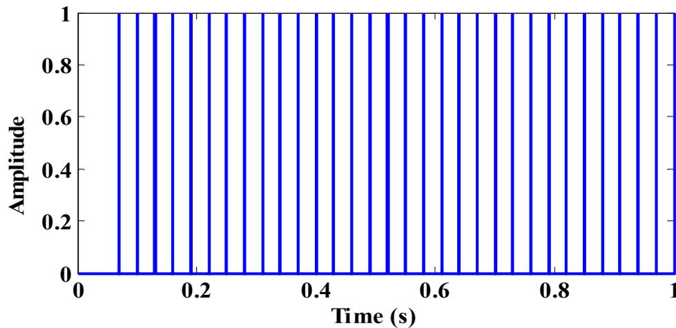
*Fig. 6 Simulated gating signals to boost converter.*
