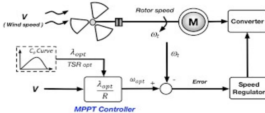
Fig. 7 Tip speed Ratio control
