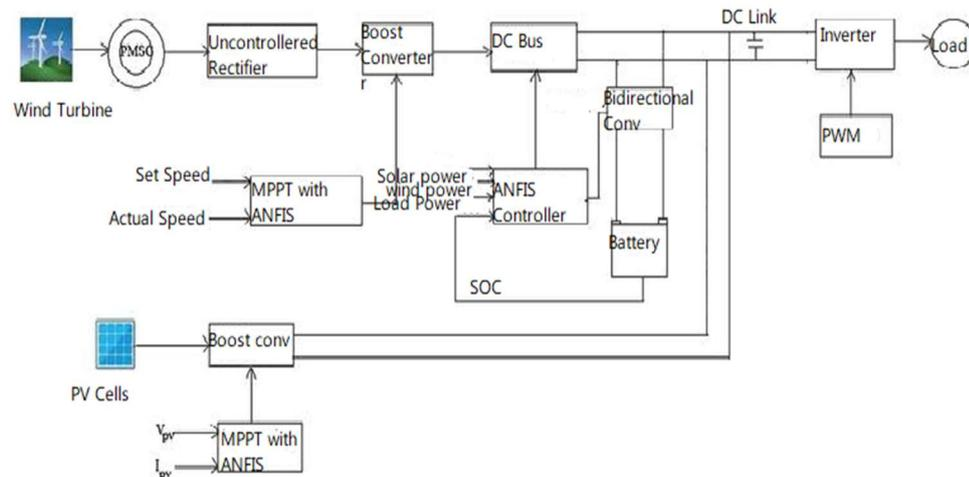
**Fig.3 Block diagram of the proposed ANFIS based MPPT.**
